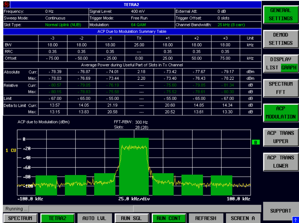
Fig. 20 ACP Due to Modulation Results (example)
