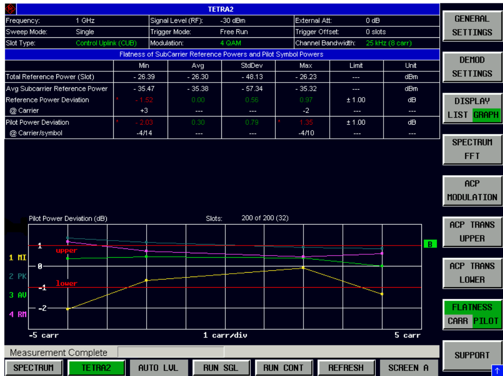
Fig. 24 Flatness measurement (example): Pilot Symbol Power Deviation
