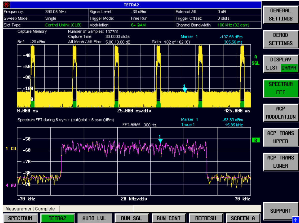
Fig. 19 Spectrum FFT Results (example)
