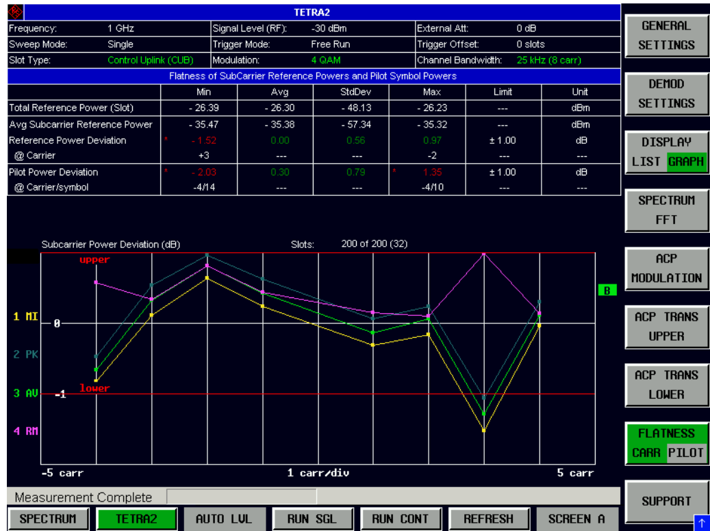
Fig. 23 Flatness measurement (example): Subcarrier Power Deviation
